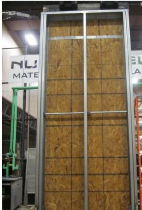
Figure 4: Oriented strand board sheathed cold-formed steel shear wall test specimen of the experimental work by Liu et al. (2014).
