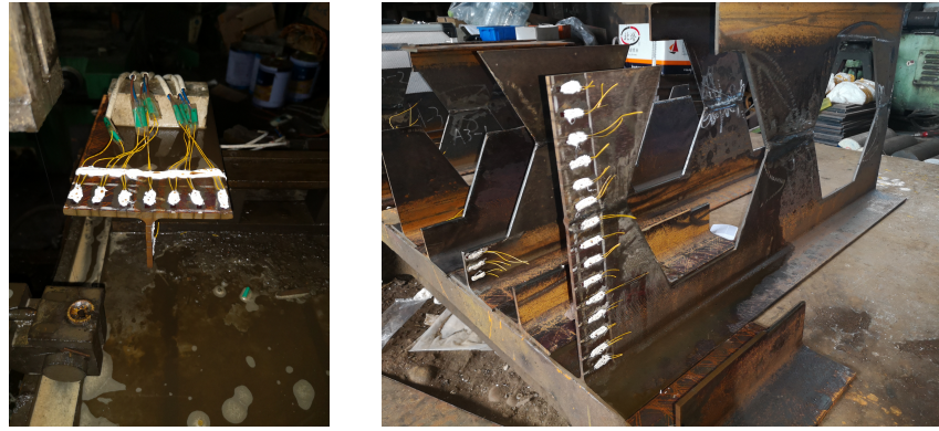
(a) the flange (b) the web after welding Figure 17: strain gauge locations for measuring residual stresses of the castellated beams
