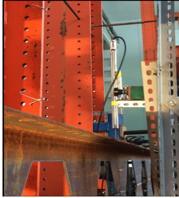
(a) displacement transducer at \frac{1}{4} span (b) displacement transducer at \frac{1}{2} span Figure 7: Vertical displacements measurement at \frac{1}{4} and \frac{1}{2} span of the beam
