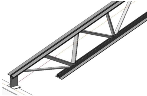
Figure 3. Geometry of open web steel joist (Vulcraft 2020).
