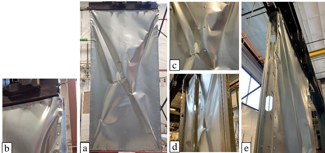
Figure 7: Failure phenomenon of Group 2 shear walls, (a) Sheet buckling after loading; (b) Sheet tearing; (c) Screws pulling-over; (d) Rear view of screws pulling-over; (e) Buckling on boundary studs
