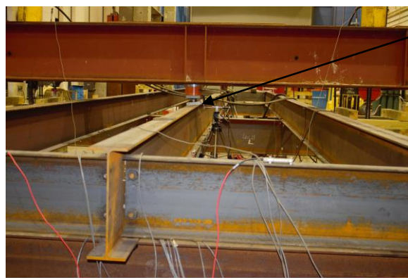
Fig. 7. LTB of the interior stringer, Test Run #3
