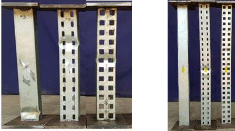
Figure 3: Failure mode of L1 and L4 specimens
