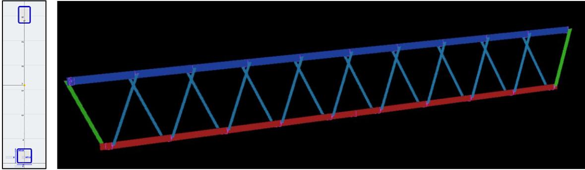
Figure 5: Hybrid 1 Design chord cross-section and joist rendering, respectively
