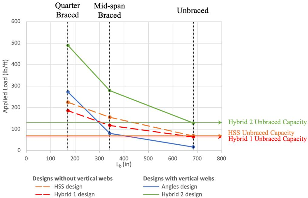
Figure 12: GMNIA distributed gravity load capacity as a function of unbraced length with self-weight
