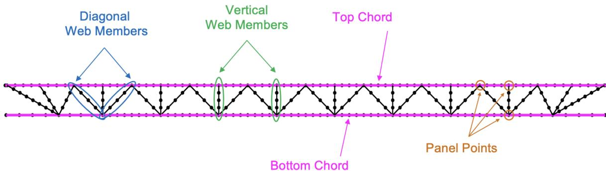
Figure 2: Open web steel joist geometry
