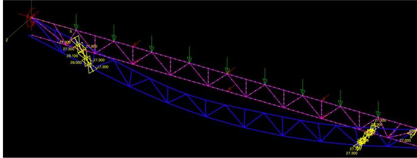
Figure 10: Web member yielding of the quarter braced Hybrid 2 Design
