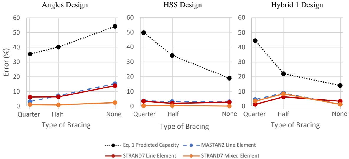
Figure 8: Comparison of linear buckling analysis for different finite element models
