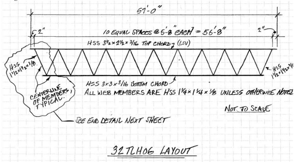
Figure 15: Geometric Properties of the HSS Design (Armbrust, 2020)
