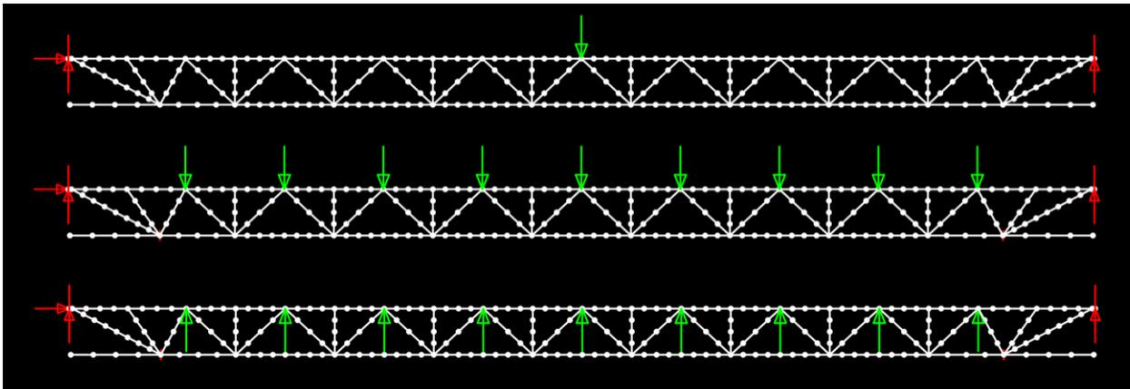
Figure 9: Point load, distributed gravity load, and distributed uplift load, respectively
