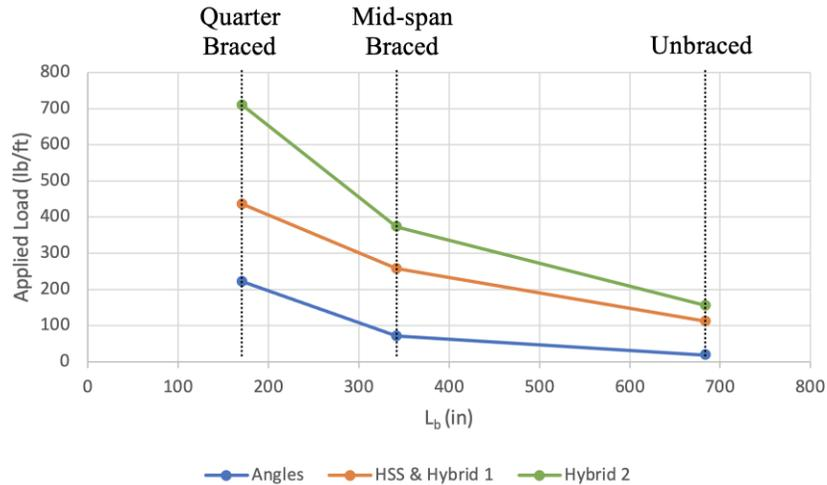
Figure 7: Anticipated joist capacities using Eq. 1 for various unbraced lengths
