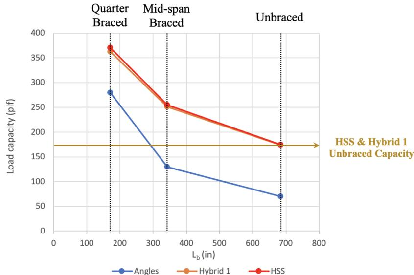
Figure 13: LBA uplift capacity as a function of unbraced length with self-weight
