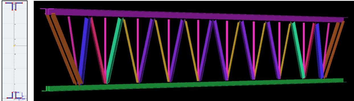
Figure 3: Angles Design chord cross-section and joist rendering, respectively
