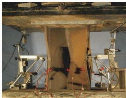
Figure 2: Local buckling mode observed in stub column. (Shi et al., 2015)
