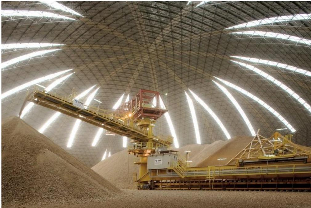
Figure 1: Interior view of the ring stockpile dome in Merida (Geometrica Inc., 2008)
