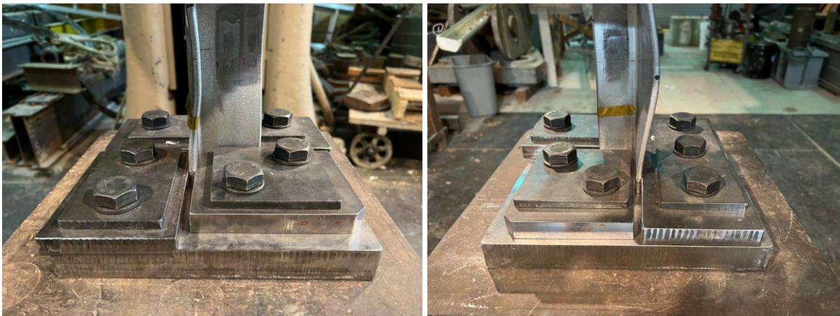
Figure 6: End plates used to achieve fixed boundary conditions
