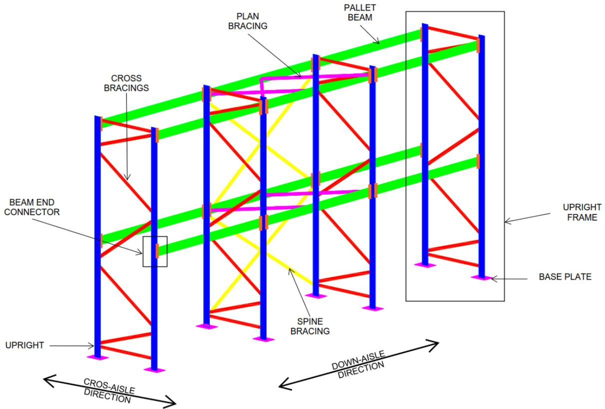
Figure 1: General arrangement of a storage rack
