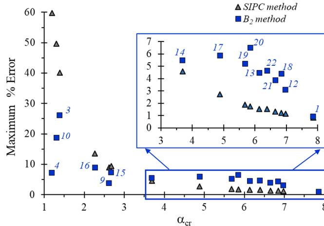
Figure 3: Comparison of the performance of SIPC and  $B_2$  methods in computing interstory drift ratios, relative to  $\alpha_{cr}$ , for the 16 applicable frames (Ziemian and Ziemian 2021a).
