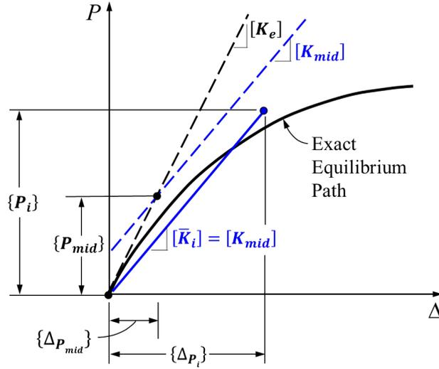
Figure 1: Graphical representation of the single increment predictor-corrector (SIPC) solution scheme
