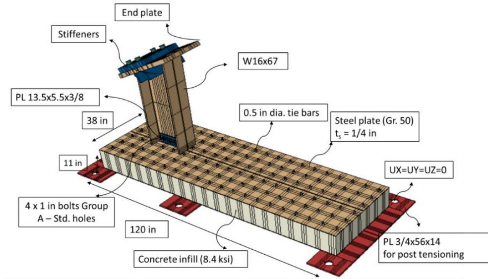
Figure 7: 3D model of the floor-to-SpeedCore wall connection
