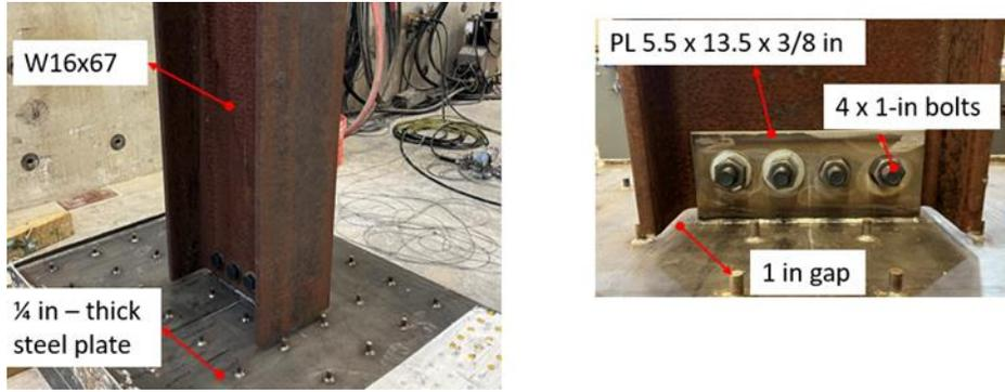
Figure 2: The size and dimension of the beam and connection components
