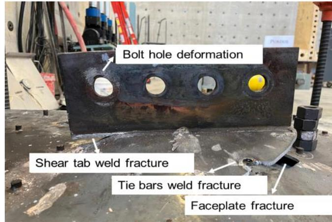
Figure 6: Failure observations during the loading test (ambient)
