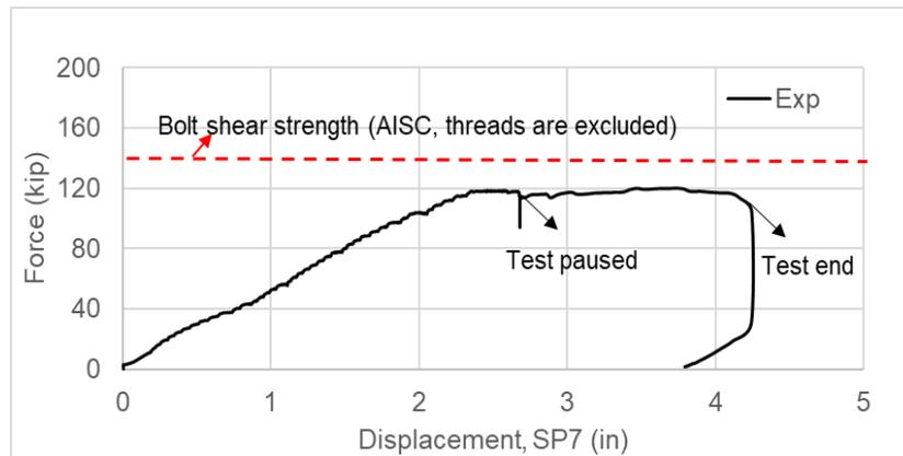
Figure 5: Connection response during the loading test (ambient)
