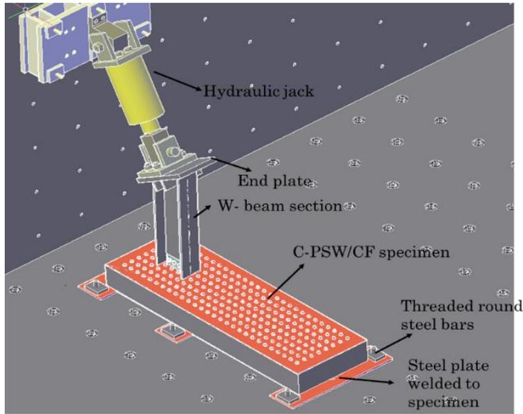
Figure 3: 3D CAD drawing of the test setup and the specimen
