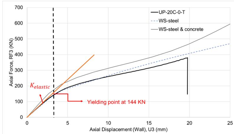
Figure 14: Comparison of the specimen model and the plate spring models
