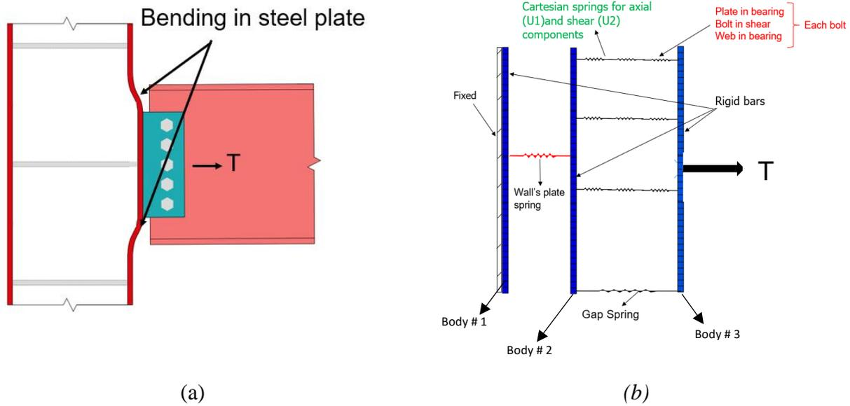
Figure 11: Schematic diagram of (a) representative of 3D floor-to-SpeedCore wall connection, and (b) the CB model for a shear tab connection of 3 bolts
