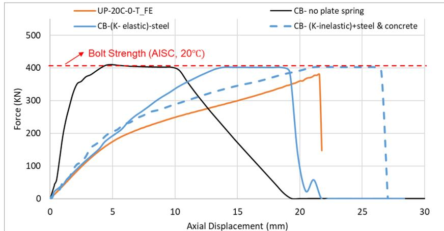
Figure 15: Comparison of detailed FE model and CB models at ambient temperature
