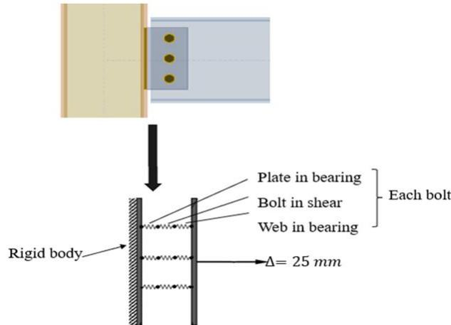
Figure 10: Schematic diagram of the model for a shear tab connection
