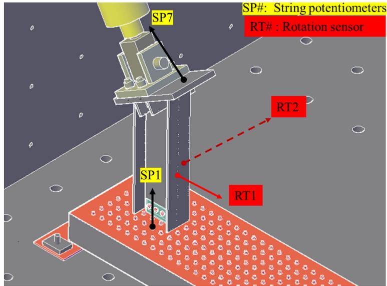
Figure 4: Instrumentations layout of the specimen
