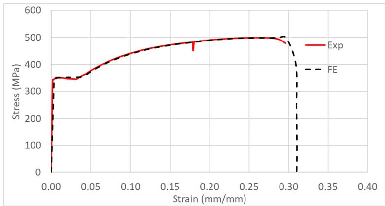
Figure 8: The comparison of the obtained results from the C-PSW/CF wall's coupon test and the FE model
