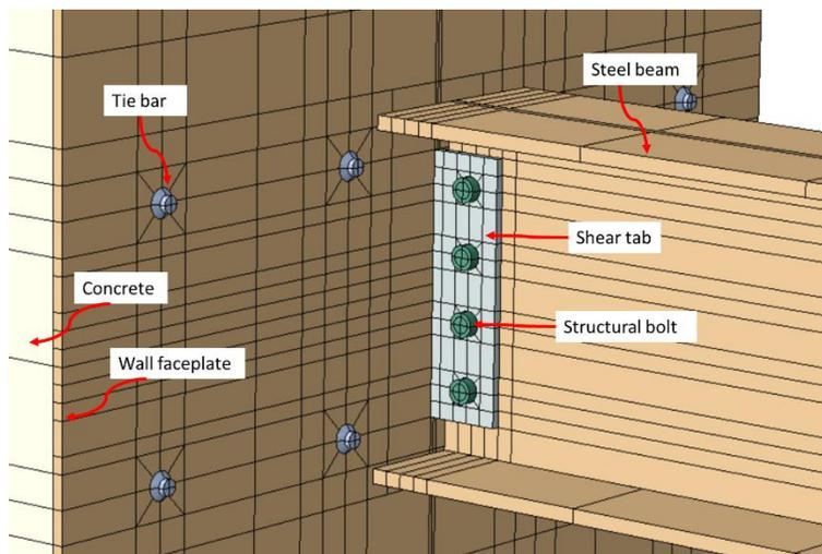
Figure 13: The detail of the connection model in the FE
