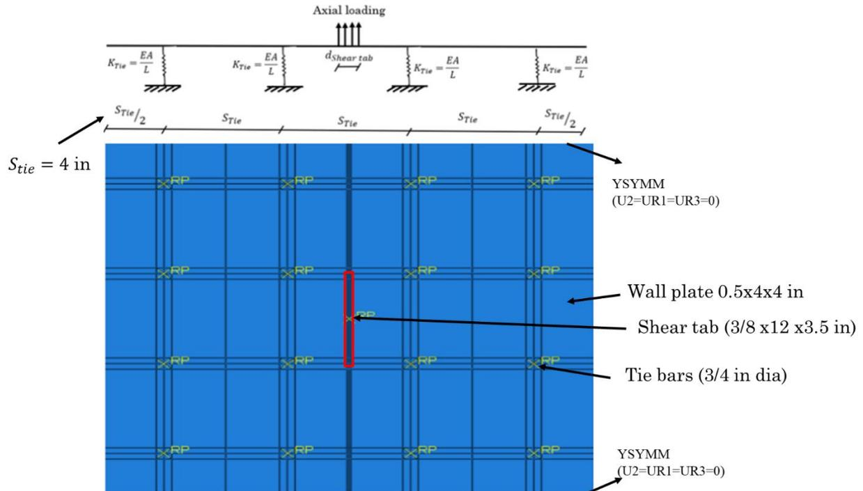
Figure 12: The wall's plate spring modeling techniques
