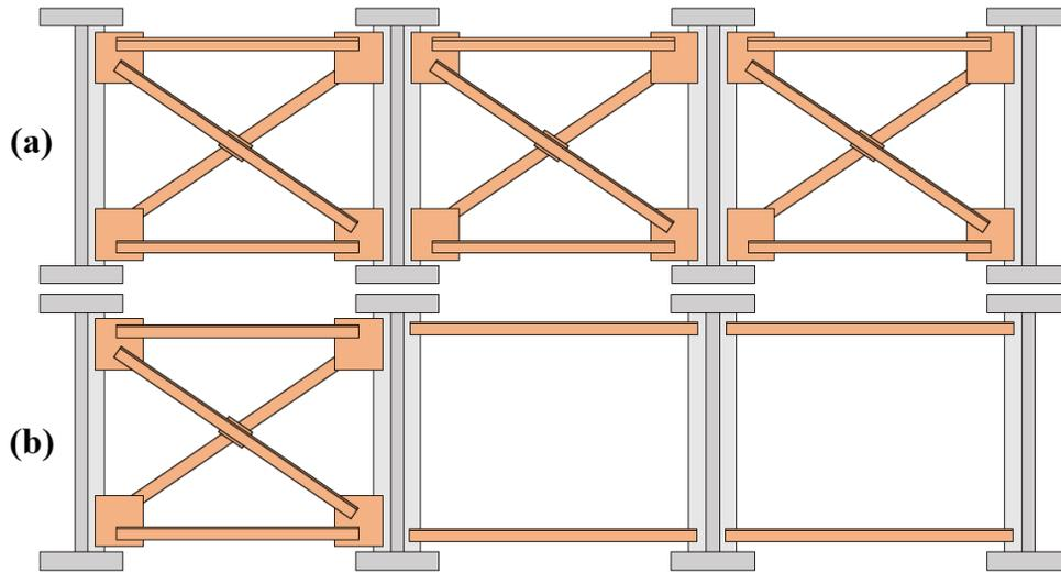
Figure 2: Example of typical bracing system with full cross-frames (a) and using lean-on bracing (b)
