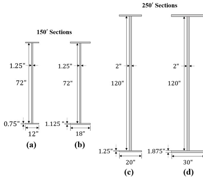
Figure 4: Illustrations of sections used for parametric study that includes a 150 ft (45.72 m) section (a/b) and 250 ft (76.20 m) sections (c/d). The left of each pair is based upon a width to depth ratio of  $1/4$  whereas the right of each pair is based upon a ratio of  $1/6$ .
