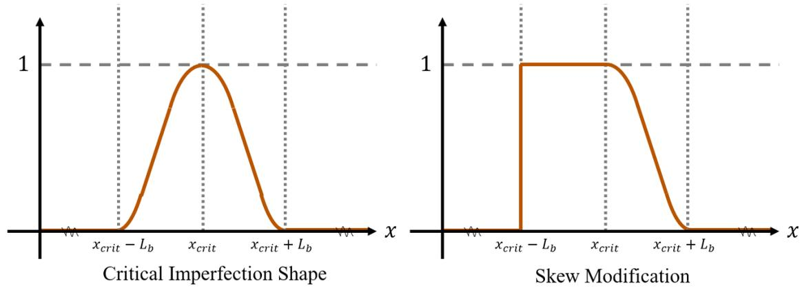
Figure 5: Illustration of critical imperfection shape produced by Eq. 5. and skew modification.
