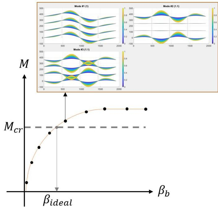
Figure 7. Example of a load-stiffness curve and the results of an included datapoint.
