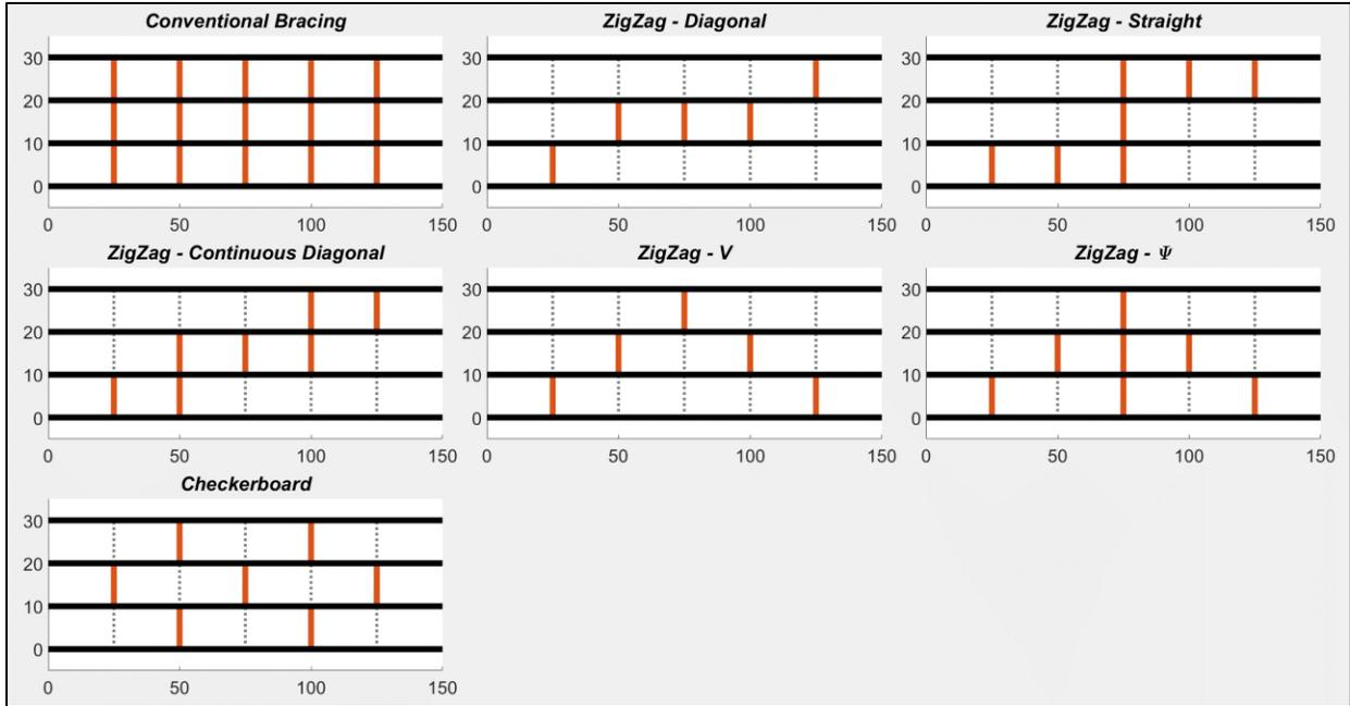
Figure 6. Cross-frame configurations utilizing lean-on bracing to be used in parametric study.
