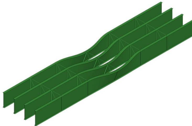
Figure 3: Exaggerated shape of critical imperfection located in maximum moment region
