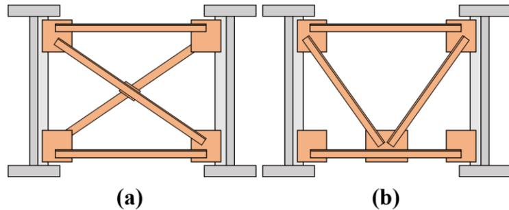
Figure 1: Examples of lateral torsional braces: (a) X-frame and (b) K-frame.
