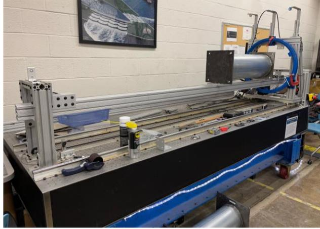
Figure 4: Laser scanner with a 250mm diameter tube
