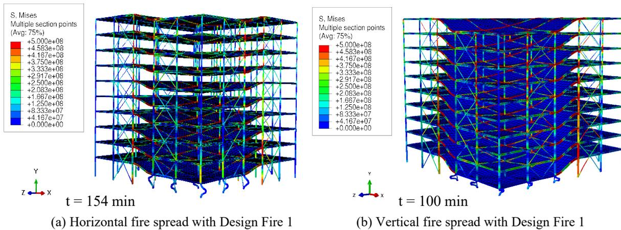
Figure 5: Deformed shape of the building under varying fire spread scenarios
