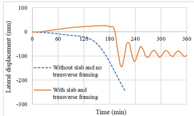
Figure 8: Effect of varying load paths on the onset of fire-induced progressive collapse
