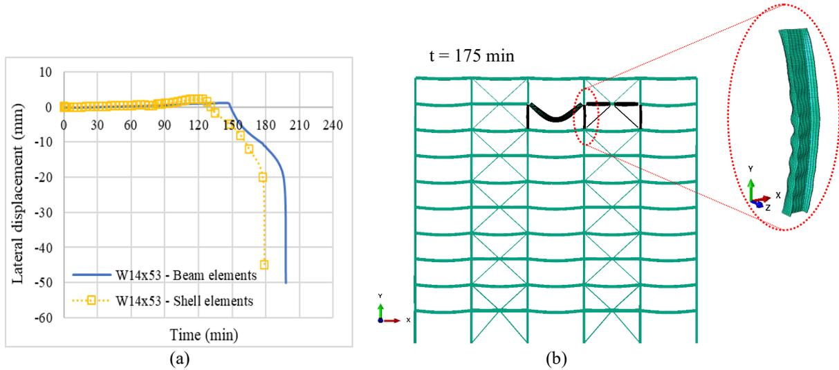
Figure 7: Effect of local instabilities on the onset of fire-induced progressive collapse
