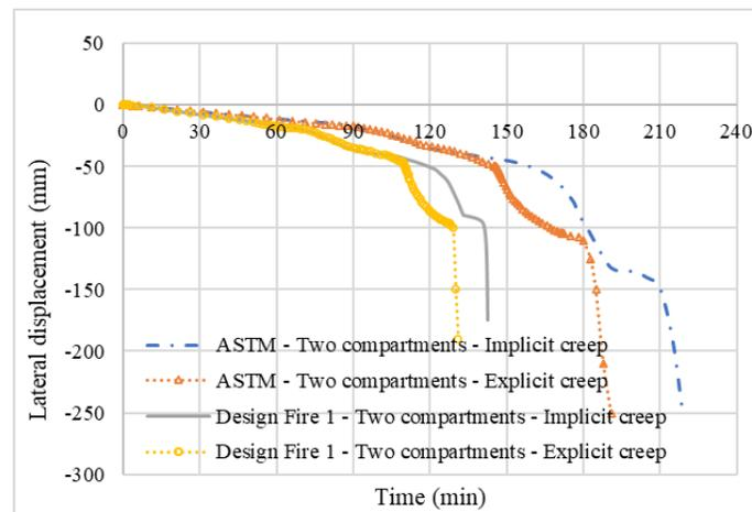
Figure 6: Effect of high-temperature creep on the onset of fire-induced progressive collapse
