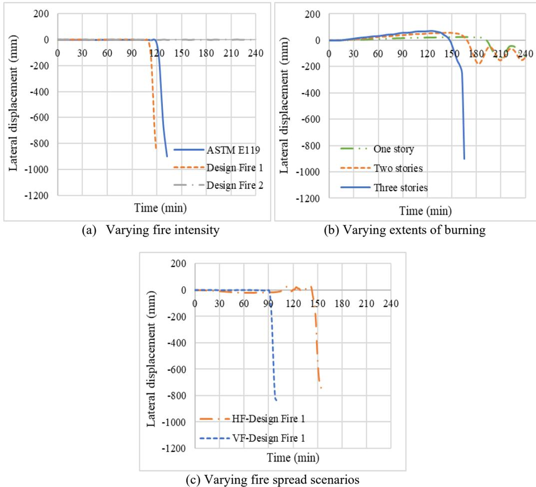
Figure 4: Effect of fire parameters on the onset of fire-induced progressive collapse
