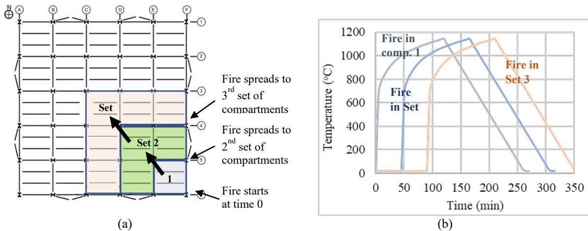
Figure 3: (a) Horizontal fire spread scenario in one story (b) Temperature-time variation in the fire-exposed compartments
