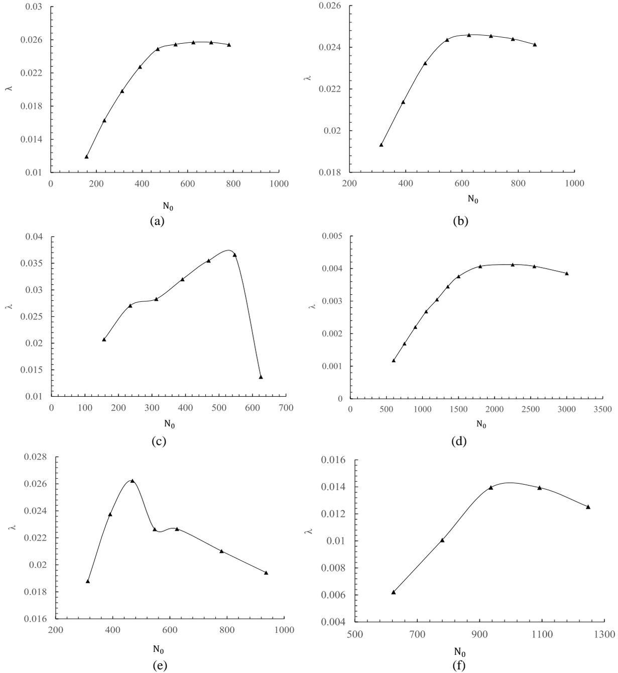
Figure 14: The variation of the parameter  $\lambda$  with the variation of  $N_0$  : (a) Schwedler monoclinal dome (b) Schwedler bidirectional (c) Radial rib dome (d) lamella dome (e) Sunflower dome (f) Hexagon dome
