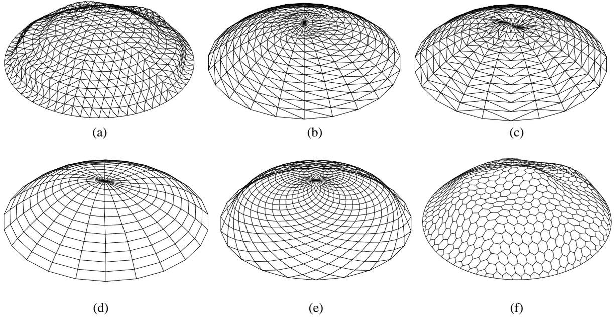
Figure 9: First buckling mode for the dome configurations: (a) Kiewitt dome (b) Schwedler monoclinal dome (c) Schwedler bidirectional dome (d) Radial rib dome (e) Lamella dome (f) Hexagon dome
