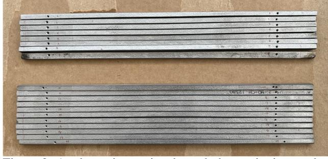
Figure 2: Angle cut into strips through the sectioning method
