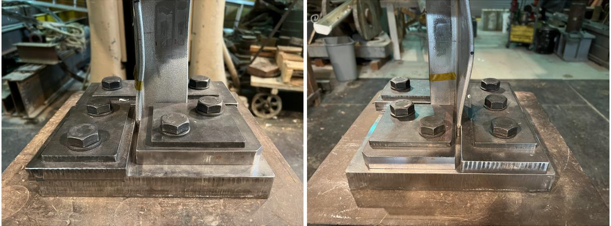
Figure 7: End plates used to achieve fixed boundary conditions
