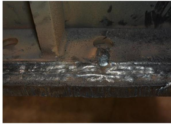
Figure 9: Bottom Flange Repair with Welded Plate of Specimen 4E-1.5-1.75-36a
