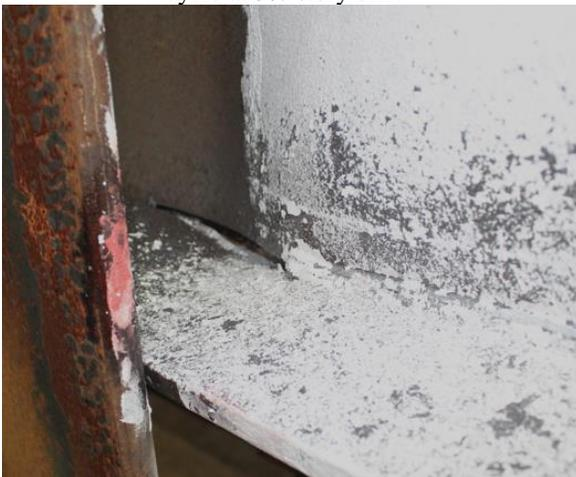
Figure 13: Fracture of Beam Web to Beam Flange Weld of Specimen 4E-1.5-1.75-36b
