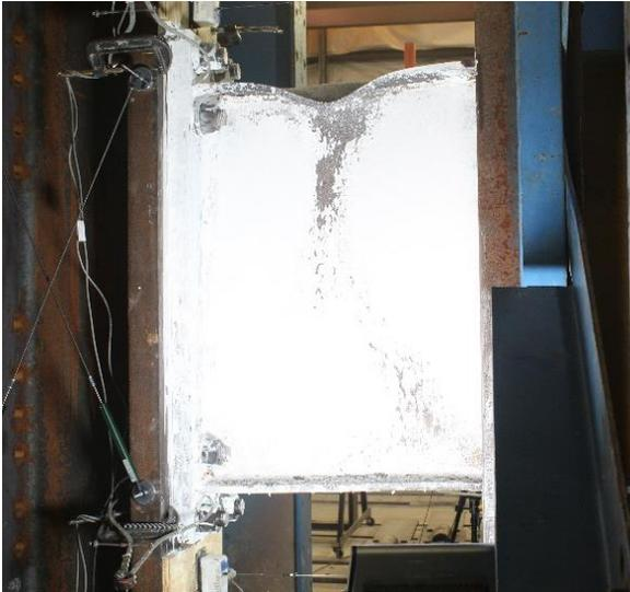
Figure 11: Flange local buckling during the first cycle at 3% story drift
