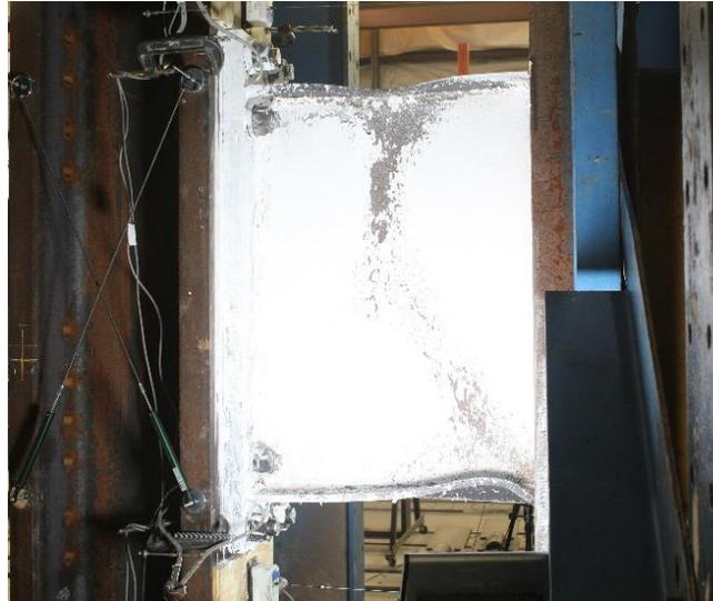
Figure 12: Beam flange local buckling extending approximately 3 ft to 4 ft from the face of the column
