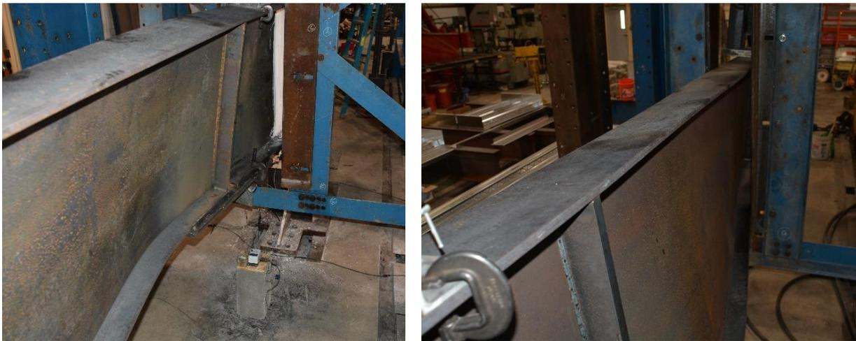
Figure 10: Lateral Torsional Buckling of the Beam of Specimen 4E-1.5-1.75-36a
