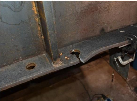
Figure 8: Bottom Flange Fracture at Bolt Holes of Specimen 4E-1.5-1.75-36a
