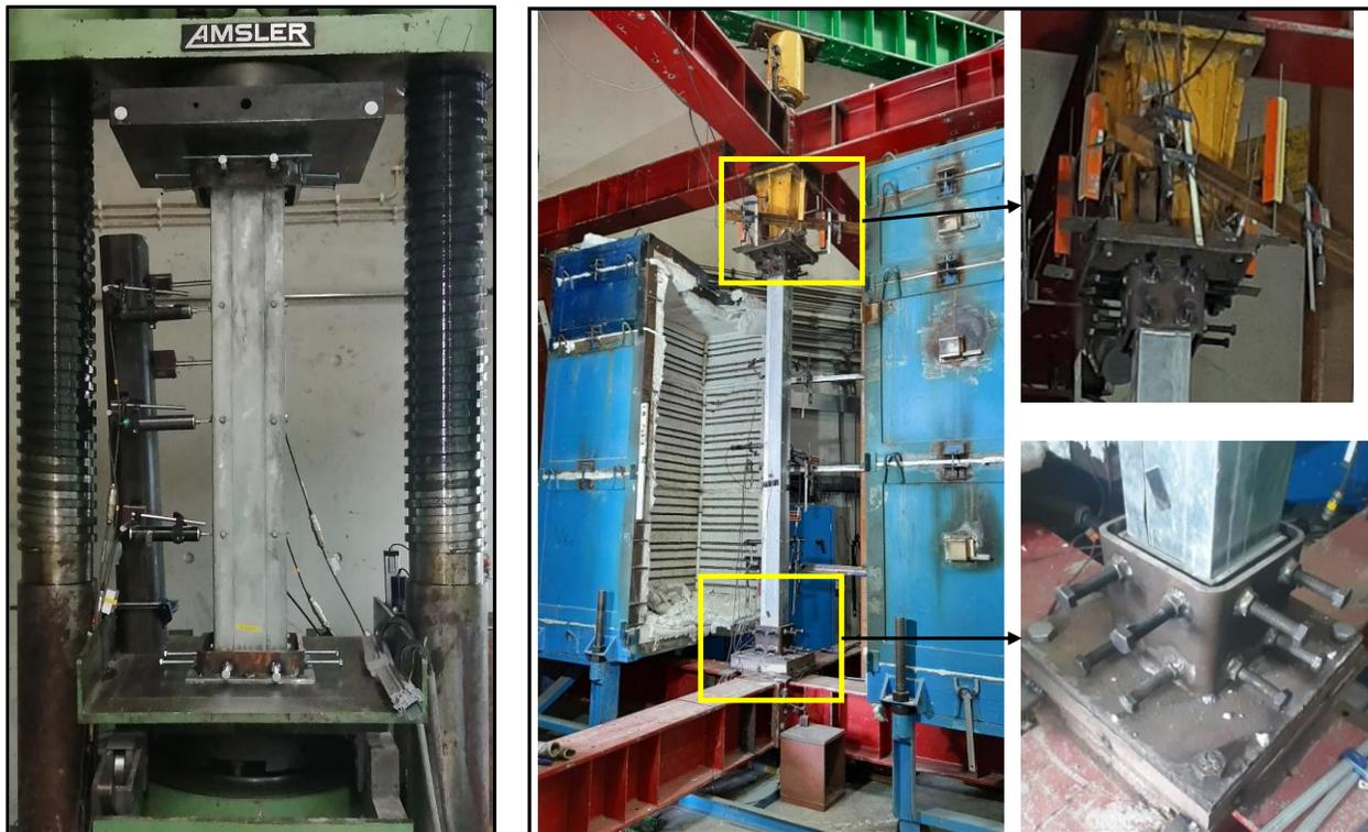
Figure 5: Test setup detail for a) short columns and b) long columns
