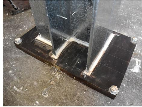
Figure 5: End plate details for a 3C120 built-up specimen: (a) dimensions, (b) actual end support after pouring Patternstone
