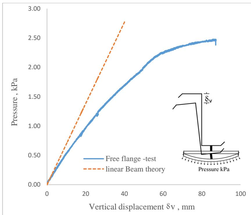
Figure 5: Pressure –vertical displacement curves of zed purlins
