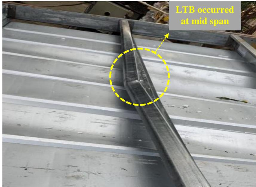
Figure 4: Failure mode of purlin
