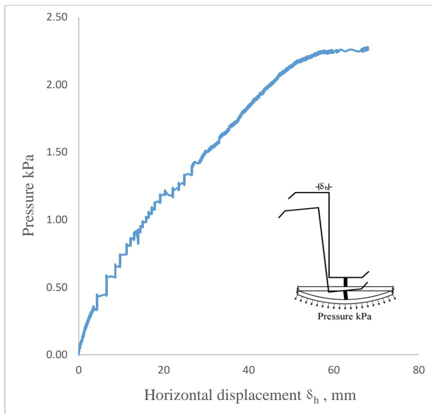
Figure 6: Pressure–horizontal displacement curves of zed purlins
