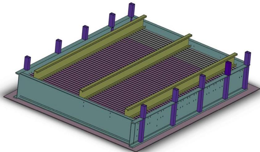
Figure 3: Test rig along with purlins and panels
