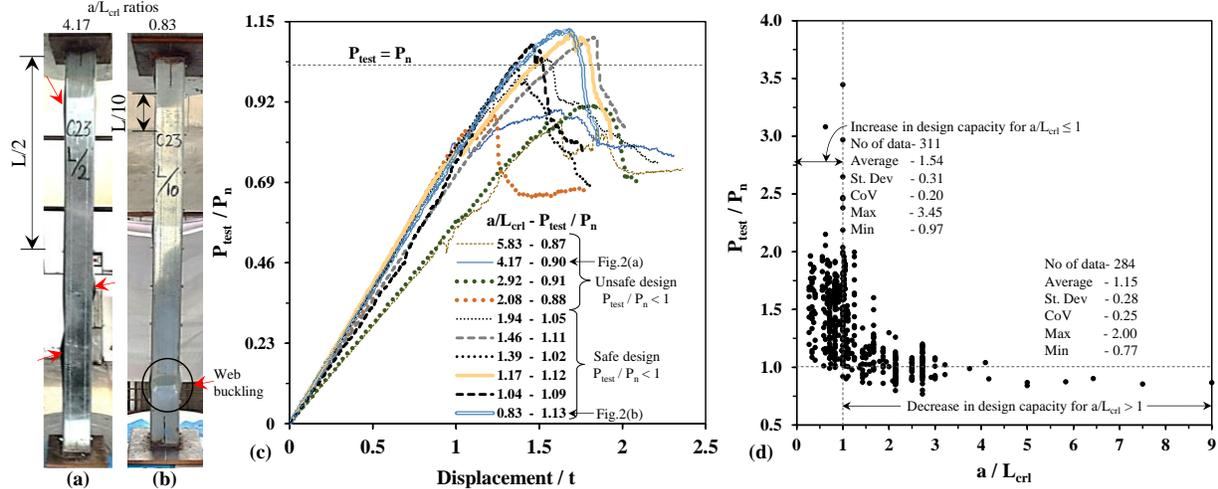
Fig. 2. Representation of built-up column test results for analyzing the influence of intermediate fastener spacing: (a) failure mode of column with  $a/L_{cr1}$  ratio of 4.17; (b) failure mode of column with  $a/L_{cr1}$  ratio of 0.83; (c) load displacement response with a design results for built-up columns of various  $a/L_{cr1}$  ratios; (d) collective data: comparison of column test and design results with  $a/L_{cr1}$  ratios
