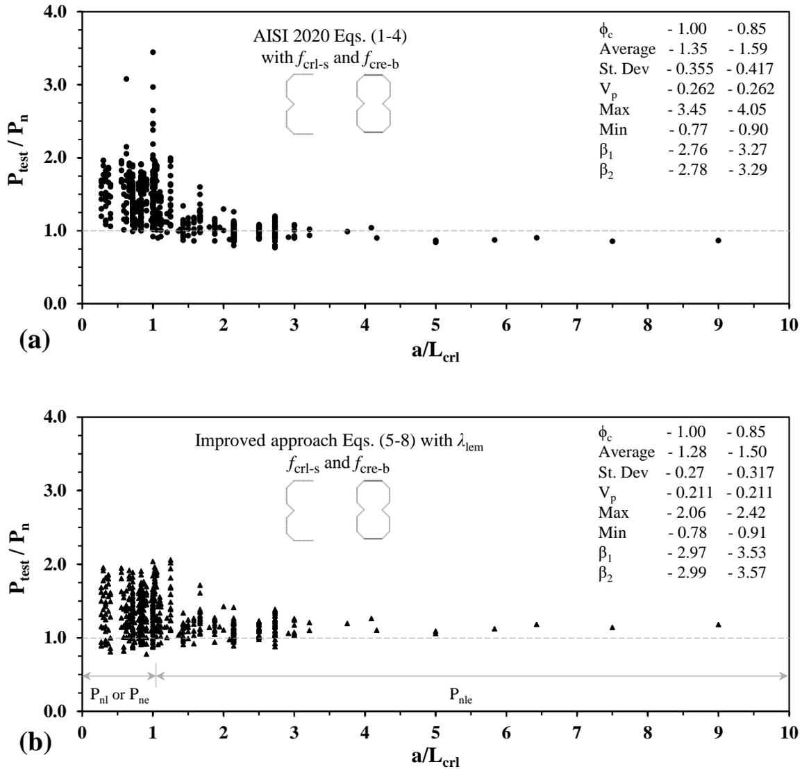
Fig. 3. Distribution of design predictions using various approach with respect to  $a/L_{crl}$  ratio: (a) original DSM (current version) from AISI (2020); (b) Improved DSM approach (Eqs. 1-4 - with  $f_{crl-s}$  and  $f_{cre-b}$ )
