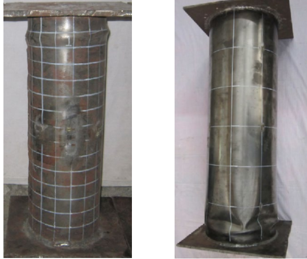
Figure 1: CHS failure modes. (a) Elephant foot failure (b) Diamond shape pattern (Guo et al., 2016).
