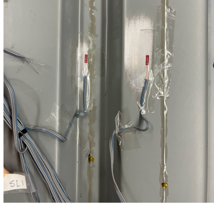
Figure 6: Fiber optic cables and strain gauges at SLB1 and SLT1
