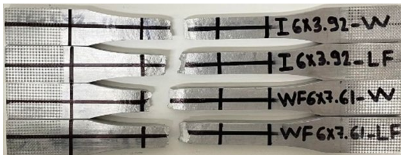
Figure 4: Tested tensile coupons for I and H sections
