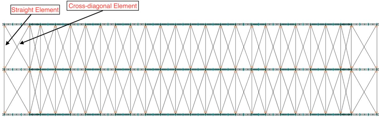
Figure 9: Deck diaphragm truss elements modeled in MASTAN2.
