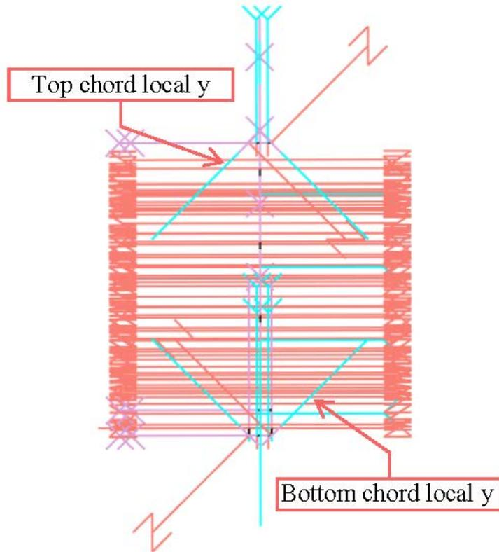
Figure 6: Side view of the joist indicating chords orientation (Red = Local z axis, Cyan = Local y axis, Purple = Local x axis).
