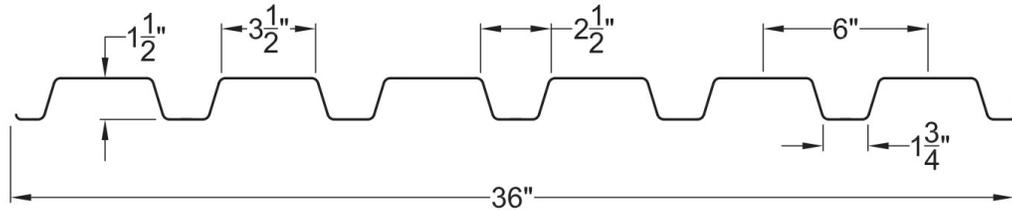
Figure 8: Deck profile utilized in the model (D-MAC-Industries, 2023).
