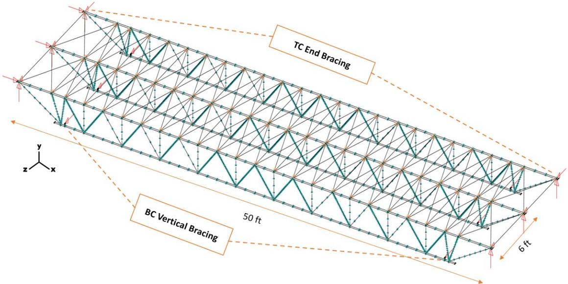
Figure 1: End model layout of the system (red is boundary conditions, orange is member ends fixity, and light blue is nodes meshing).
