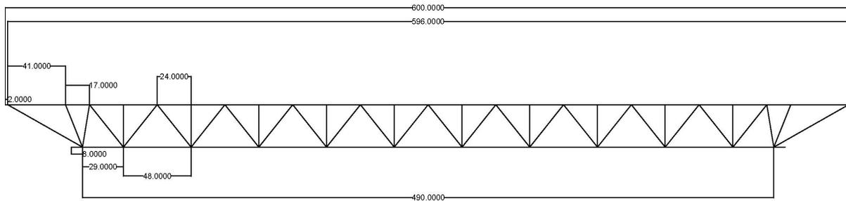
Figure 3: End model layout of the Joists (all dimensions are in inches).
