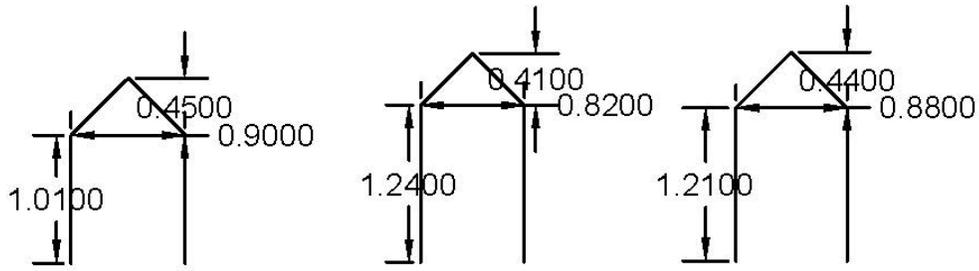
Figure 5: Modeled crimping section, from left to right, represent crimping for L  $1.25 \times 1.25 \times 0.109$ , L  $1.5 \times 1.5 \times 0.17$ , and L  $1.5 \times 1.5 \times 0.123$ , respectively (all dimensions are in inches).
