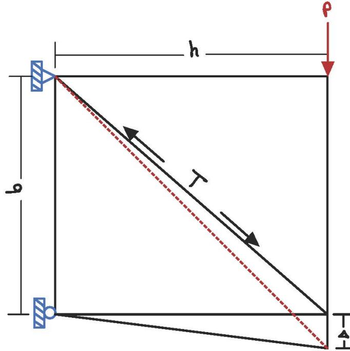
Figure 10: Truss sample highlighting the main dimensions utilized in deck modeling truss elements method .
