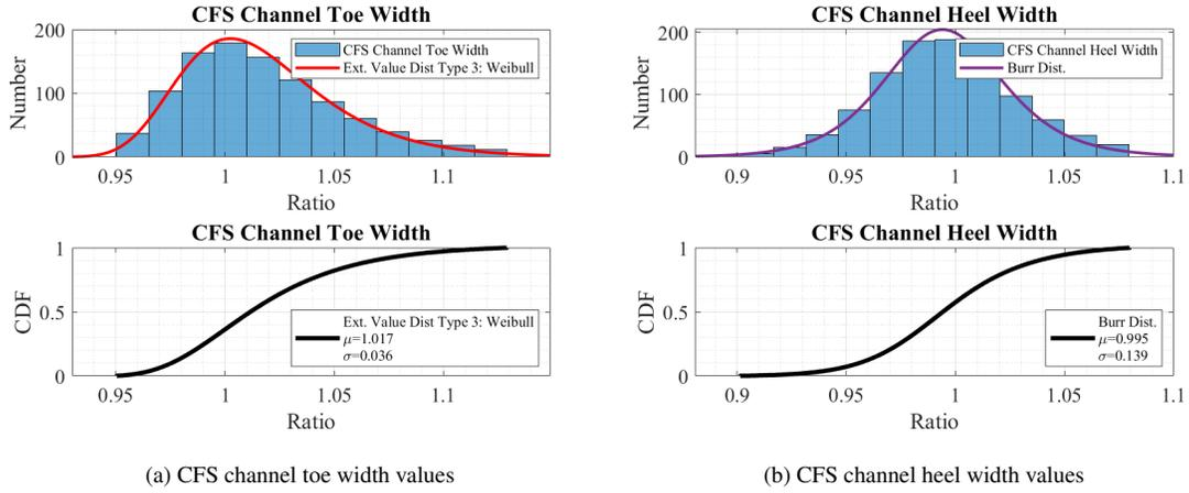
Figure 12: Histogram and statistical parameters of generated random CFS cross-sectional width values
