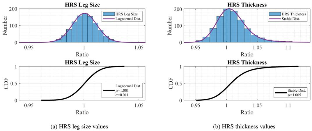
Figure 10: Histogram and statistical parameters of generated random HRS cross-sectional values
