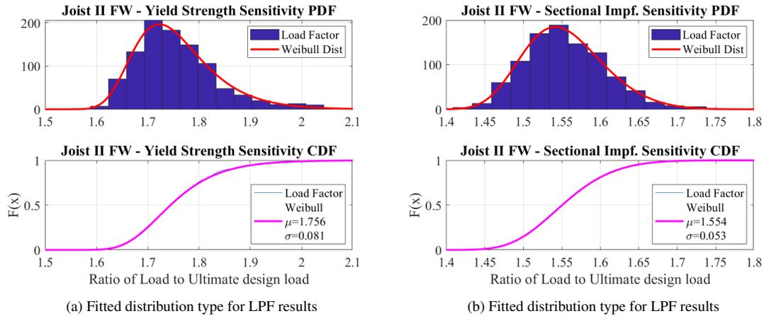
Figure 20: Joist II FW sensitivity analyses results and fitted distributions
