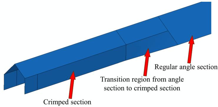
Figure 6: HRS angle web crimped at 6 inches at the ends (Cicek, Sputo, and Blum, 2024)
