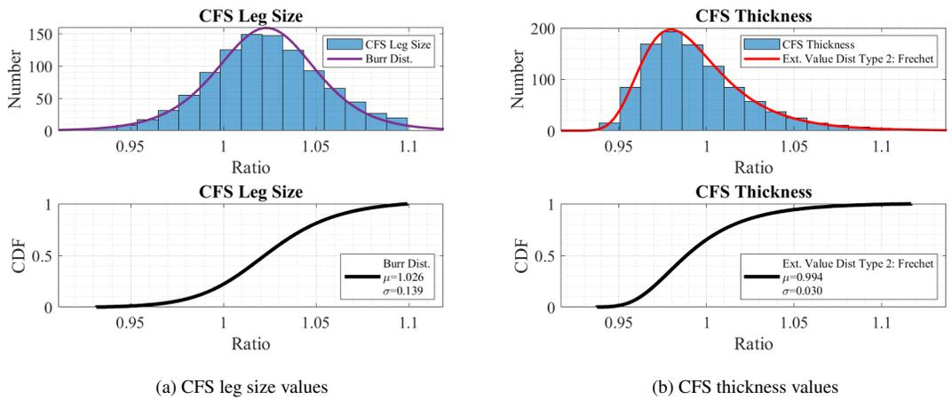
Figure 11: Histogram and statistical parameters of generated random CFS cross-sectional values
