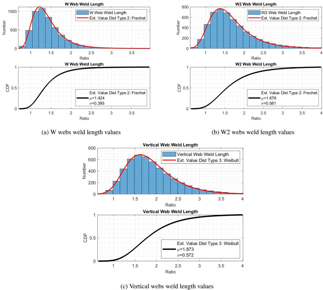
Figure 13: Histogram and statistical parameters of generated random weld lengths values
