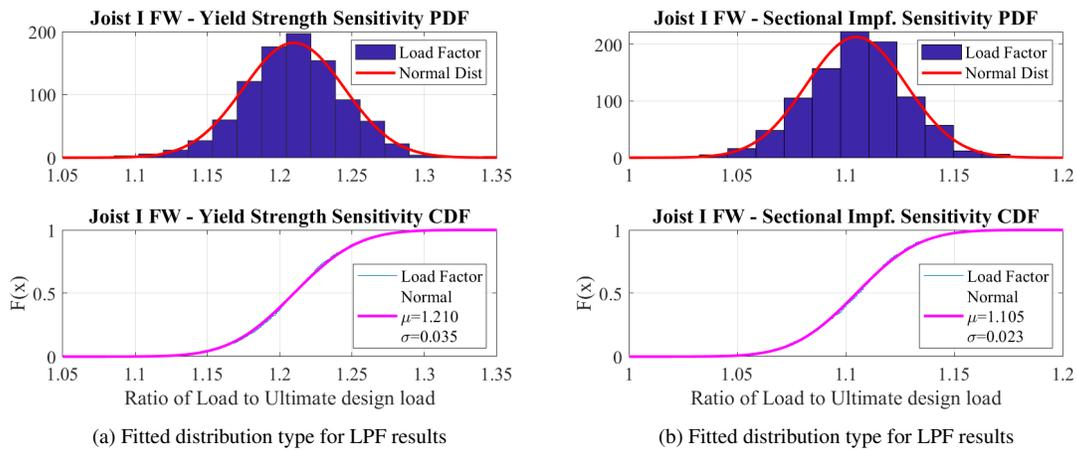
Figure 17: Joist I FW sensitivity analyses results and fitted distributions
