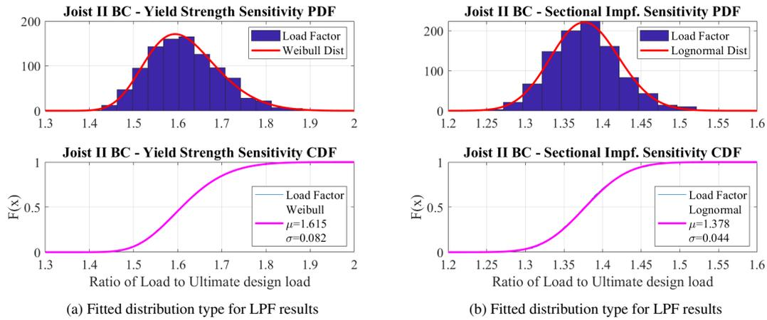
Figure 19: Joist II BC sensitivity analyses results and fitted distributions
