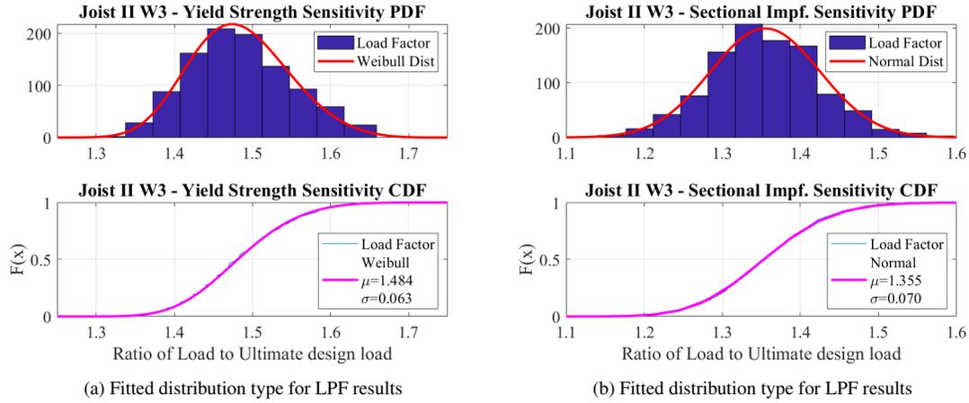
Figure 21: Joist II W3 sensitivity analyses results and fitted distributions
