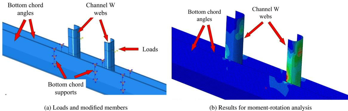
Figure 7: Modified shell element models for web rotational stiffness calculations (Joist II)
