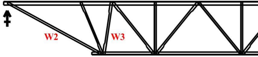
Figure 1: Joist with HRS sections (Joist I)
