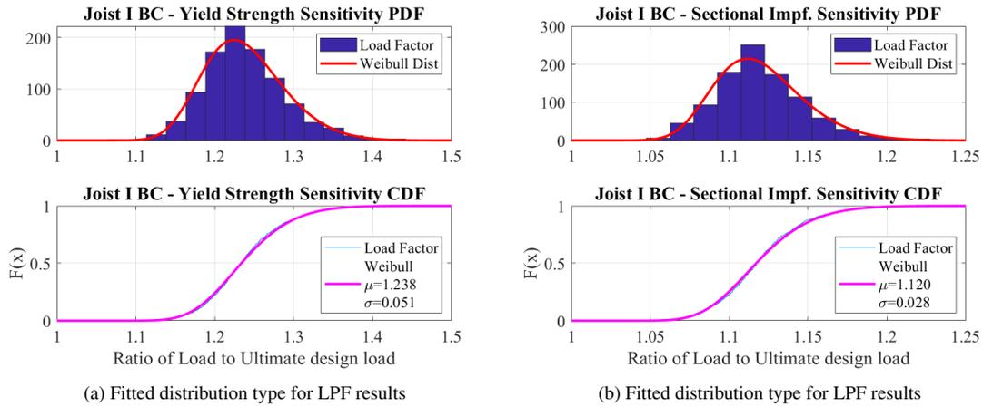
Figure 16: Joist I BC sensitivity analyses results and fitted distributions
