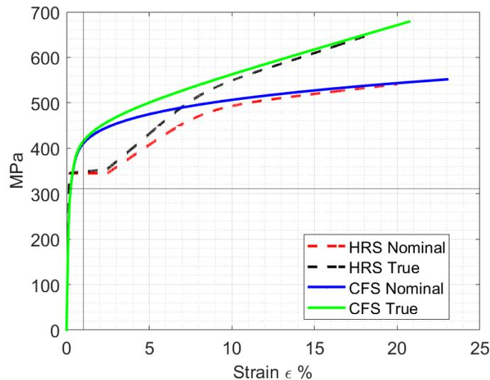
Figure 4: Material models for HRS and CFS sections
