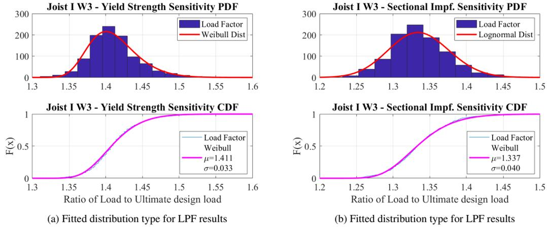
Figure 18: Joist I W3 sensitivity analyses results and fitted distributions
