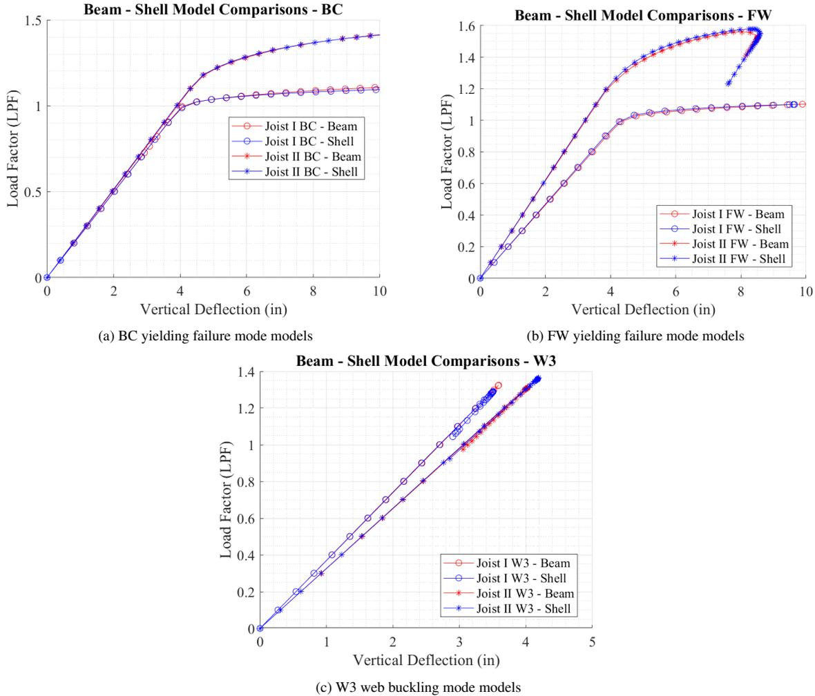
Figure 8: Load - Deflection curve comparison for beam and shell element FE models
