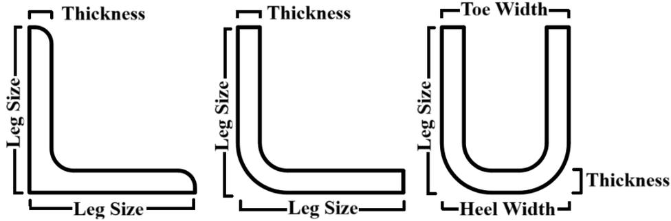
Figure 3: Left: HRS angle, Middle: CFS Angle, Right: CFS Channel sections
