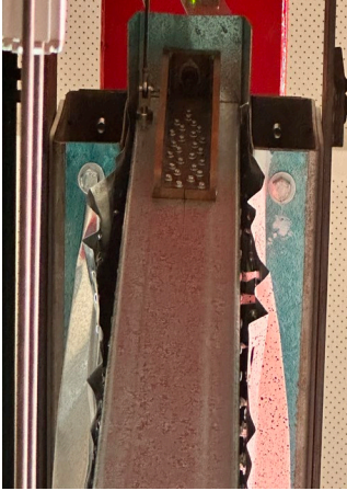
(a): Separation of sheathing from the frame on both sides
