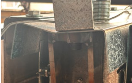
(b): Bearing and tear-out failures of the sheathing
