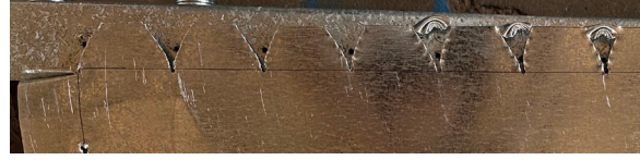
(b): Bearing and tear-out failures of the sheathing
