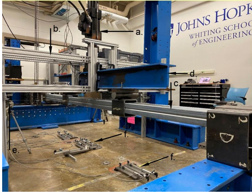
Figure 5. Minor axis bending test setup with lips in tension (LIT): a. actuator, b. aluminum frame, c. specimen, d. spreader beam, e. lateral PTs, f. ground PTs
