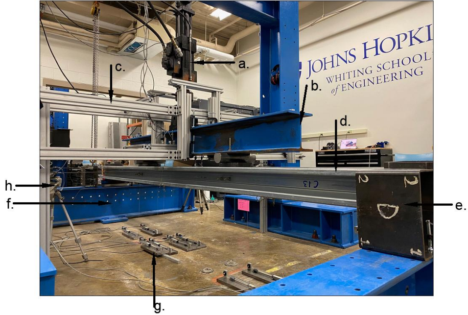
Figure 7. Annotated picture of major axis bending test setup with no steel panels: a. actuator, b. spreader beam, c. aluminum frame, d. specimen, e. lateral supports, f. end beam support, h. cameras
