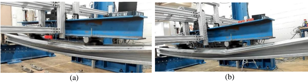
Figure 17. Post failure images from the major-axis tests without steel deck panels: (a) Major-1, (b) Major-2, (c) Major-3, and (d) Actuator load-deflection plots (continued)
