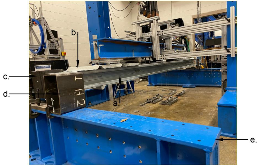
Figure 9. Major axis bending test setup with steel decks in the shear spans: a. specimen, b. steel panels, c. 7 \times 7 \times 1/2 HSS sections, d. lateral supports, e. end beam support
