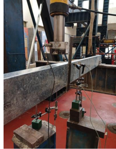
c) Load application and LVDT's
