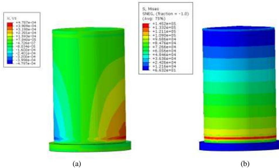
Figure 9. (a) deformation (m) response of Tank, and (b) Von-mises stresses (Pa).
