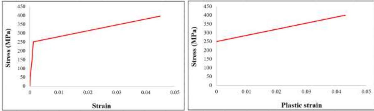
Figure 4. Bi-linear stress and strain relationship of steel
