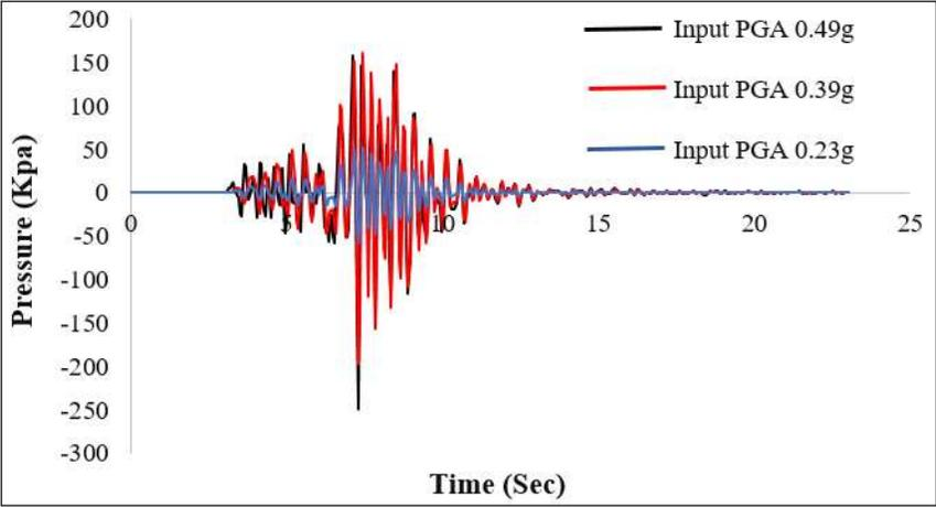
Figure 17. Comparisons of total hydrodynamic pressure (Kpa) vs time response under different input PGAs
