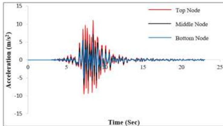
Figure 14. Time history response of Tank under Friuli earthquake
