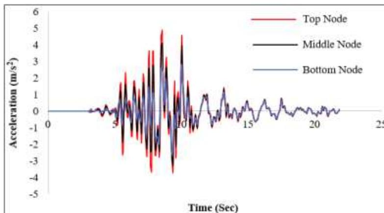
Figure 15. Time history response of Tank under Emeryville earthquake
