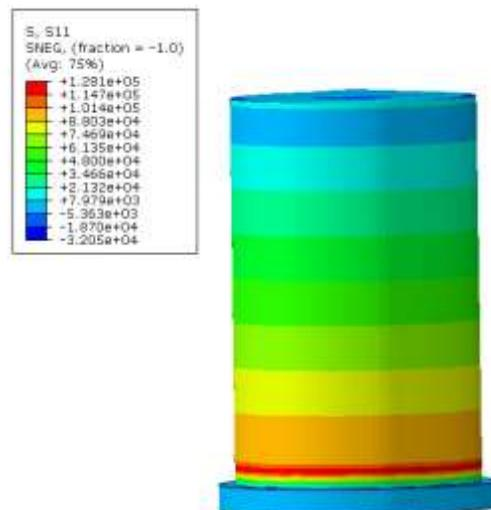
Figure 10. hoop stresses at Tank wall (Pa).
