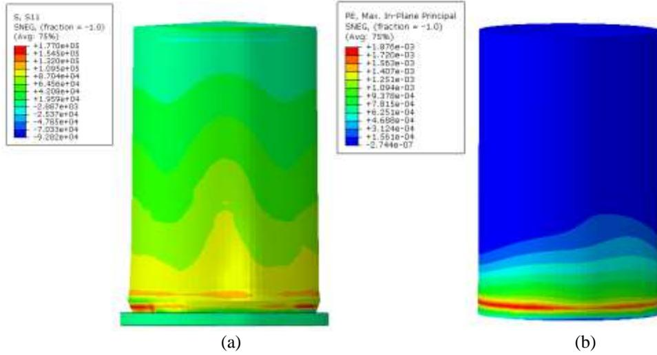
Figure 12 (a). Circumferential stress (Pa), and (b). Max. tensile strain
