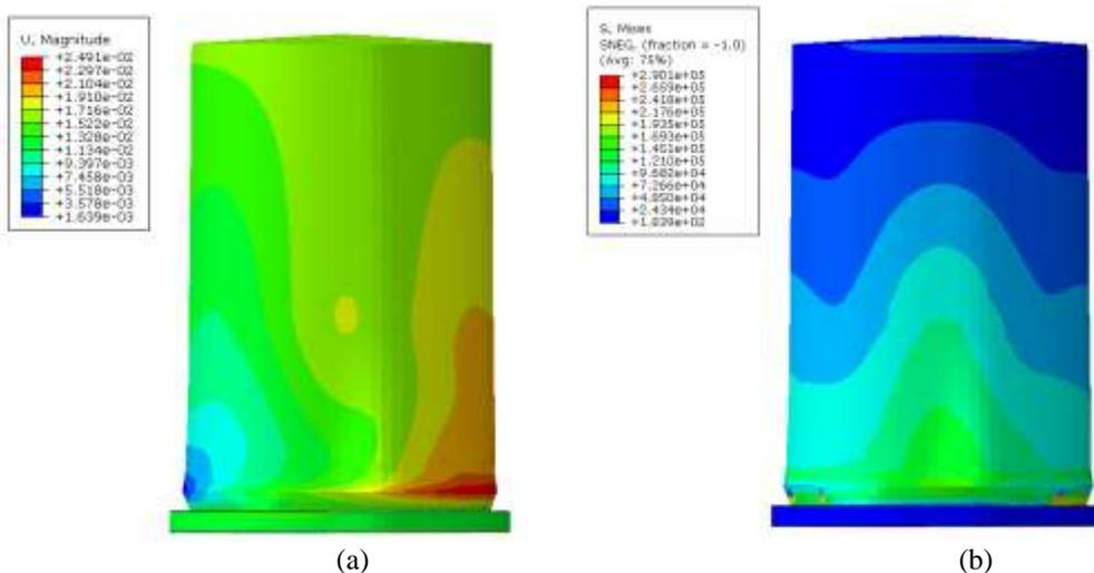
Figure 11. (a) Deformation (m), and (b) Von-mises stress distribution (Pa)
