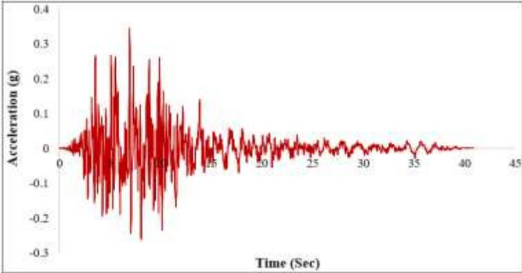
Figure 7. Input time history-Kobe earthquake.
