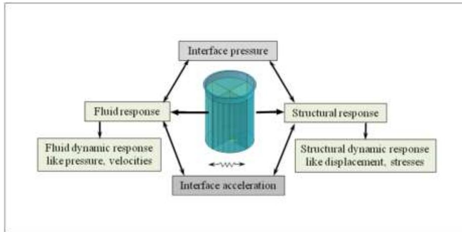
Figure 3. Fluid-structure interaction in liquid-filled tank
