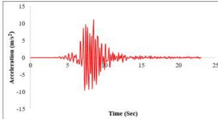
Figure 13. Time history response of Tank under Friuli earthquake
