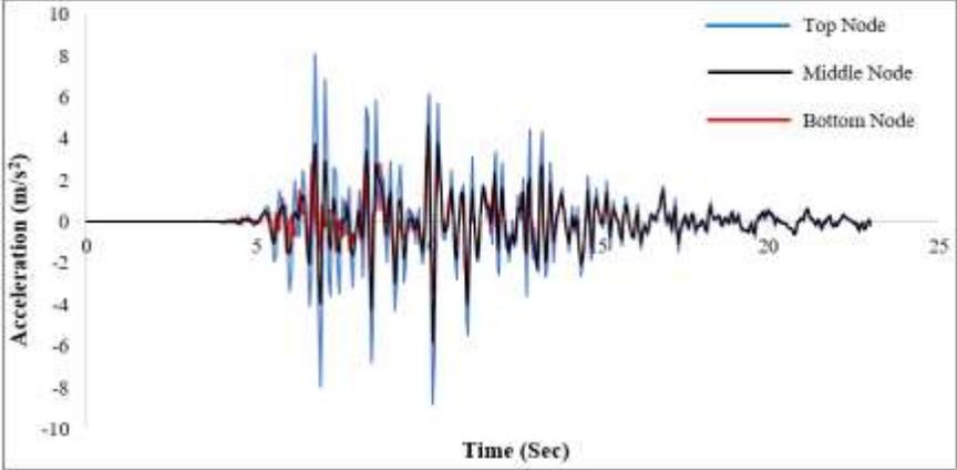
Figure 16. Time history response of Tank under Kobe Japan earthquake
