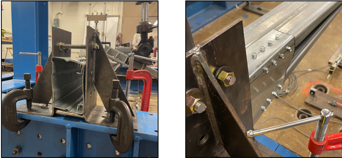
Figure 8: Observed shear deformations of the studied section at the supports of test setup #1.
