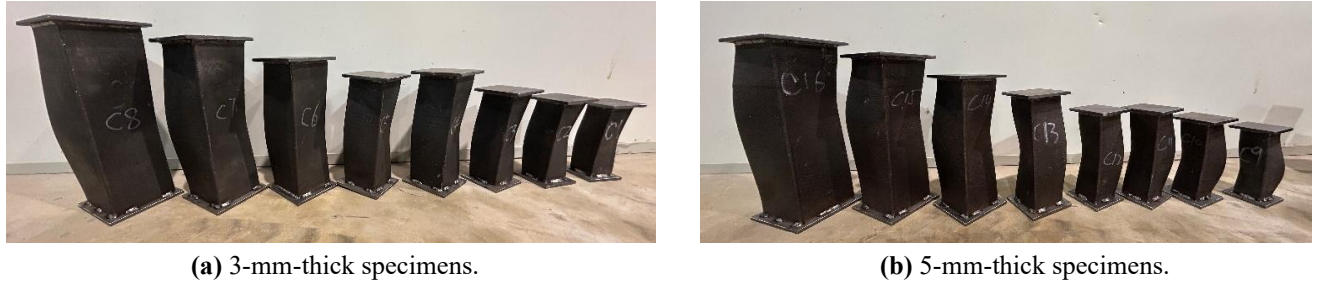
Figure 5. Failure mode of all tested WLAM lipped angle stub columns.
