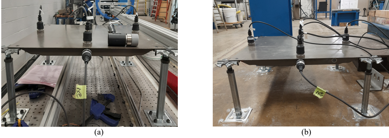
Figure 3: Experimental setup of the RAF module with accelerometers (a) RAF module fixed to the optical table using bolts (b) RAF module fixed to the floor using seal bond 95 adhesive
