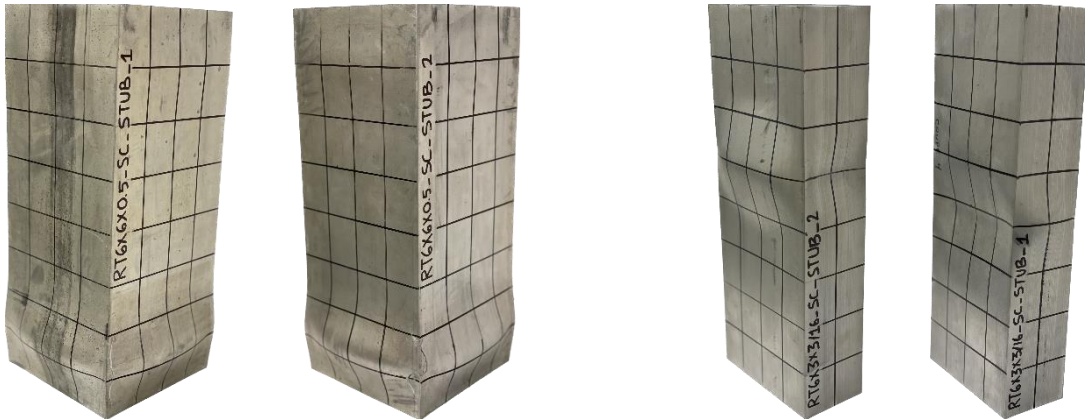
Figure 4. Stub columns deformed shapes: RHS (left) and SHS (right).
