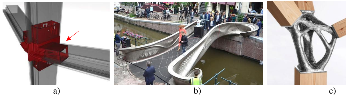
Figure 1: Landmark application of WAAM in construction – a) Aluminum printed facade node (Strauss & Knaack, 2016) – b) Pedestrian bridge in Amsterdam (3D Metal Printing for Industrial Industry, n.d.) – c) Takenaka Connector in Japan (3D Metal Printing for Industrial Industry, n.d.)
